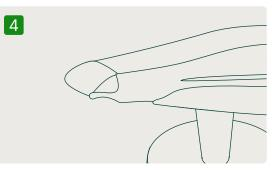
Sterilize the scanner and tips. Do **not** use CaviCide wipes on mirror tips.
